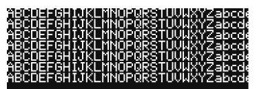
A message can also be created using **3 rows of 12.4" text**. This sized text is suitable for traffic speeds of **up to 70+ mph**.
