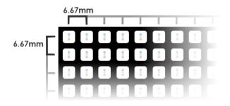
144x432 is the matrix size. This is the number of pixels high (144) and the number of pixels wide (432) of the display. That's **62,208 pixels per side!** The more pixels, the higher the clarity and amount of detail that can be shown.
