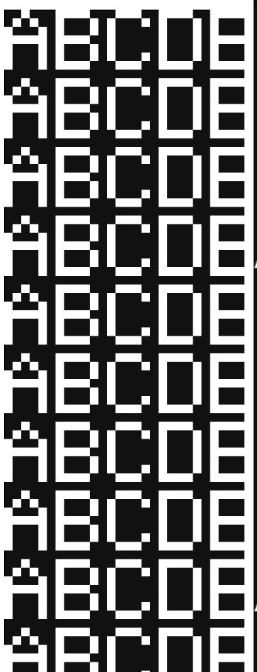
A message can also be created using **3 rows of 12.4**" **text**. This sized text is suitable for traffic speeds of **up to 70+ mph**.
